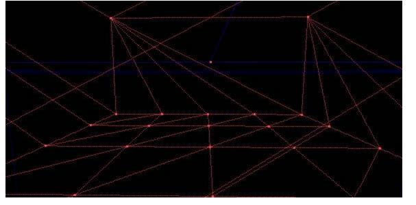
Now hold down ALT and both mouse buttons at the same time. Dragging upwards will move the vertex up, and dragging to the side will move the vertex accross the 3D view. It always moves exactly along the axis so don't worry about it moving off the grid! In the pic I moved the vertex up and left!
