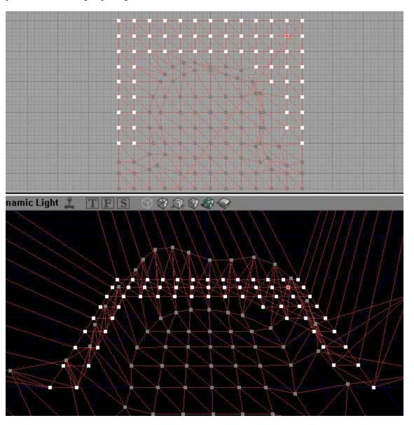
In the 3D View, hold down Ctrl and drag up with both mouse buttons to move the selected vertecies roughly up to the right height. That just reduces the amount of dragging you have to do all the time, fight that RSI!
